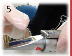
Dab the unbroken end of the fragment containing the plasma onto the refractometer surface. Be careful not to cut yourself on the sharp edges of the glass.
