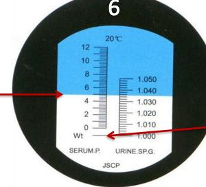
When only distilled water is placed onto the reading plate, the line should appear at this point if properly calibrated.
