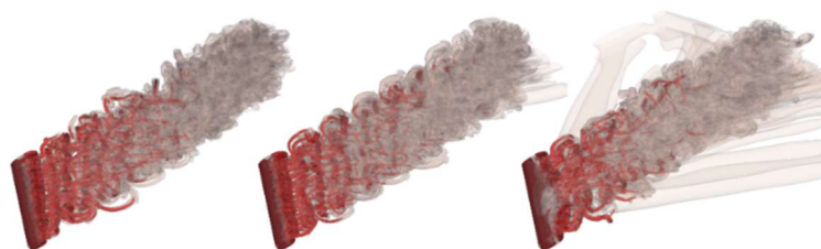
Figure 1: Vortices in the wake of the flow past a model monopile, visualized by contours of swirl strength. Panels from left to right are increasing strengths of background density stratification.
