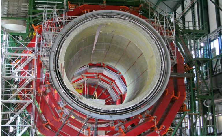
The CMS superconducting solenoid in its iron return yoke
