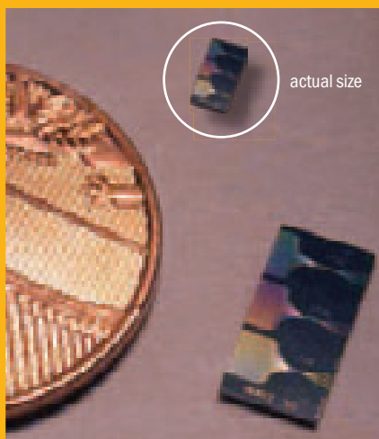
An all-optical chip developed at the University of Bristol for optical quantum computing
