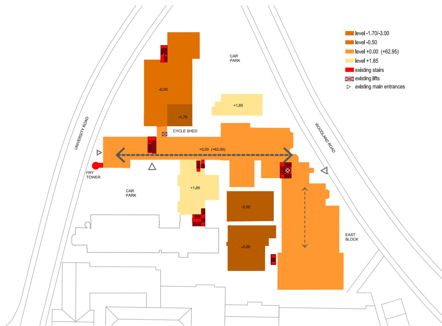
Existing Building: Circulation and Building Levels Study
