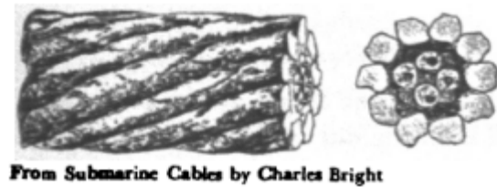
Figure 1. Piece of channel cable laid between Dover and Calais in 1851
