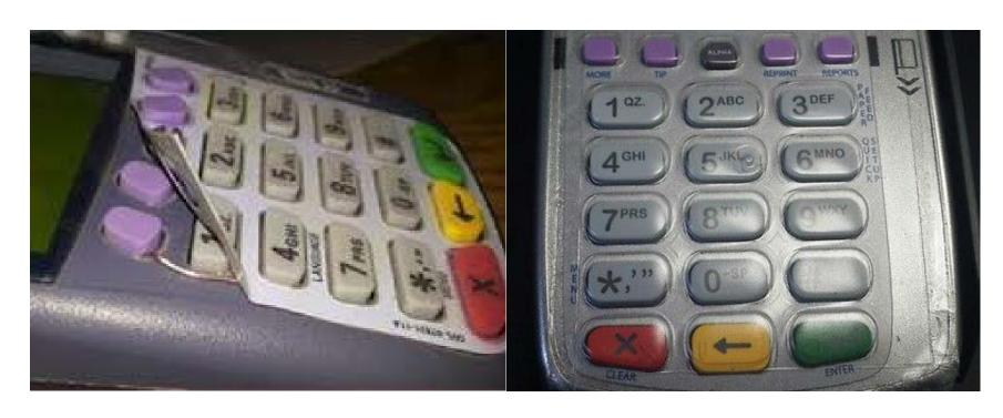
Added overlays with skimming and key-logging hardware
