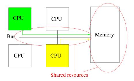
Basically a hardware problem: current multi-core architectures are not designed for timing predictability
