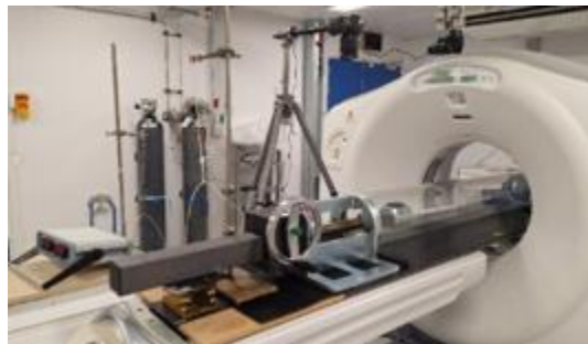
Figure 1: Tensile testing setup combines with scanner measurement
