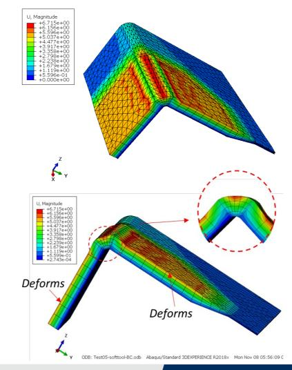
Comparison between the physical part and model prediction in defect generation
