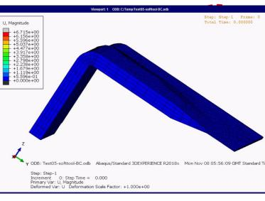
The output of the Virtual Autoclave with a representative result from vacuum bagging
