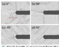
Crack length is measured from the average of the four 0 degree plies.
