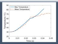
Different damage mechanisms such as fracture, damping caused by viscoelastic behaviour of the matrix or the frictional sliding between fibre-fibre and fibre-matrix interfaces cause heat generation in composites
