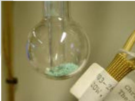
Porous metal-organic framework nanocomposites used for energy storage on-board hydrogen fuel cell vehicles
