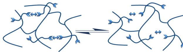
Figure 1: Concept of the elastomeric network enhanced by reversible connections. Shear - or temperature induced rearrangement.
