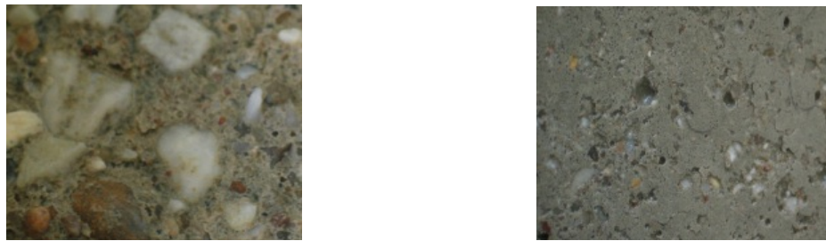
Figure 2: Image (Left). Severely carbonated slag-rich mortar surface condition after frost salt attack. Image (Right): Identical mortar with Na-MFP healing agent near surface shows almost no signs of damage under the identical frost salt attack.
