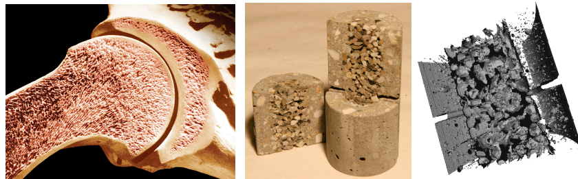
Figure 1. (a) Outer compact bone and inner cancellous (spongy) bone, (b) A new vascular concrete with porous network concrete inside apparently solid outer concrete cylinder, and (c) 3D reconstruction after x-Ray \mu CT scans.
