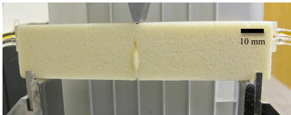
Figure 1: Photograph of healed PIR foam fracture specimen with regenerated polymeric foam material expelled from the crack plane (pMDI contained in top channel).
