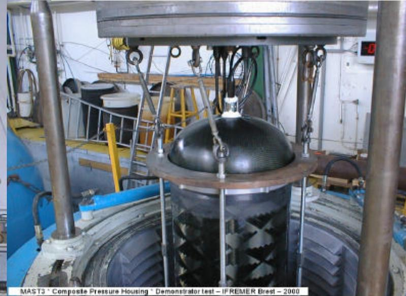
MAST3 \* Composite Pressure Housing \* Demonstrator test - IFREMER Brest - 2000
