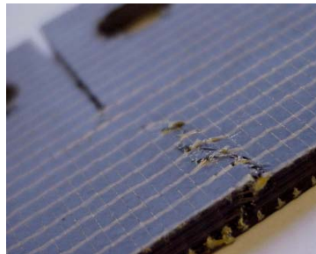
4-stack stitched 0° specimen (SS72-s0)
