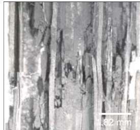
5-stack (SS69-s0) stitched 0° Brittle Response Loose Stitching
