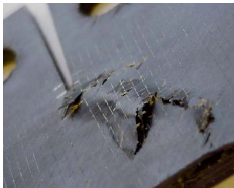
4-stack un-stitched 0° specimen (SS82-u0)
