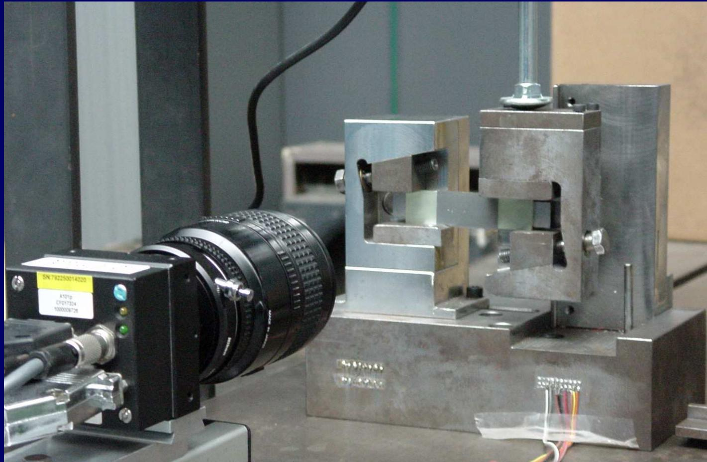
Material: 0° glass/epoxy composite (2.1 mm thick)
