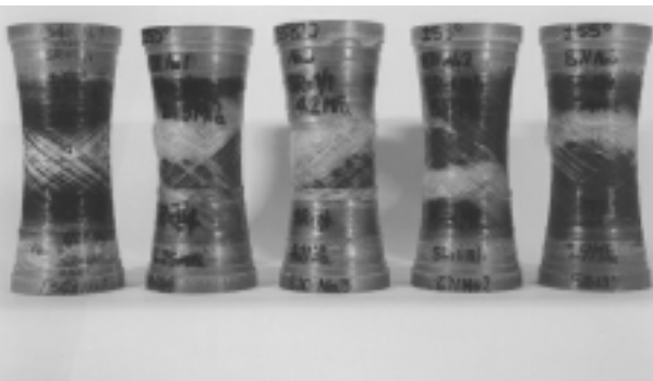
Figure 4 - A family of tubes, all manufactured in an identical manner, but tested to failure under different loading ratios.
