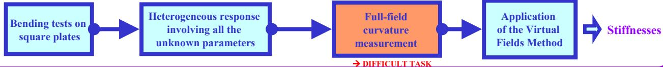
**Proposed solution: direct full-field slope measurements with deflectometry.**
