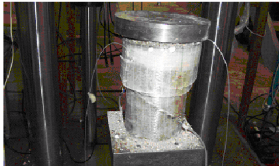
Figure 1 Compression test of GRP composite wrapped concrete cylinder with embedded EFPI and FBG sensors
