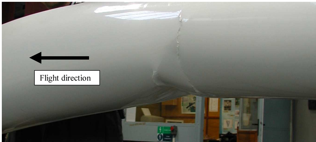
Figure 4. First failure of fuselage structure
