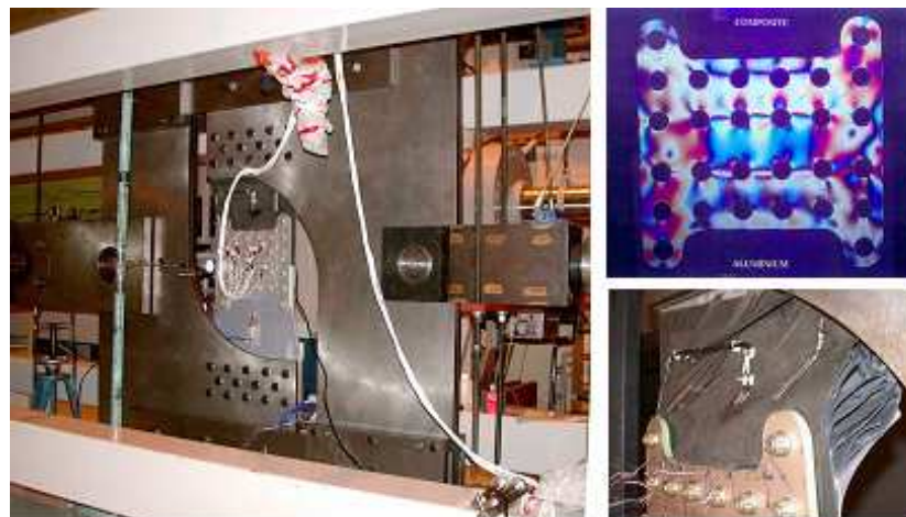
Fig 3: TANGO spar web shear test - main test (left); photoelastic under load (top right); failure (bottom right)
