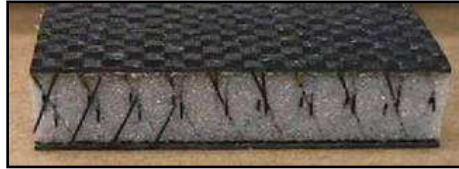
Fig.1 K-Cor™ with carbon fabric facesheets
