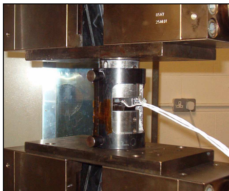
Fig. 1 Celanese Compression Fixture
