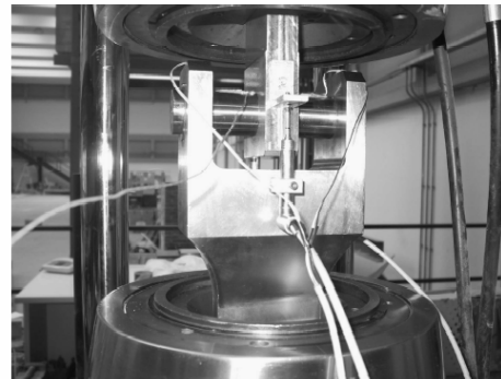
Figure 2: test rig for bending fatigue tests
