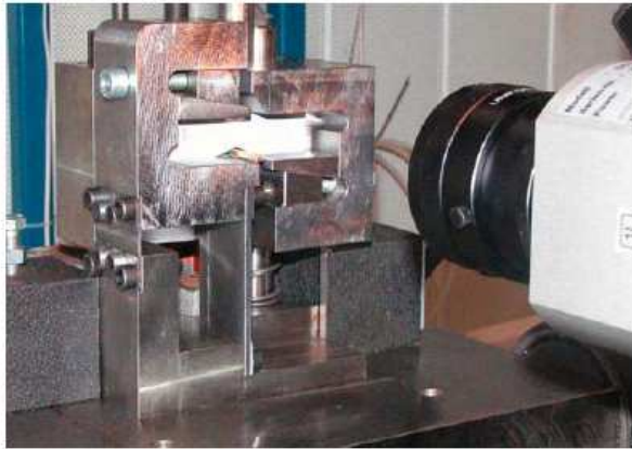
Figure 4. New Iosipescu fixture with DSP camera
