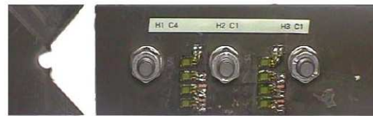
(b) Strain Gauges used for Double-Shear Joints
