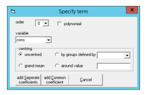
As you can see there are two options for adding terms into the multivariate model. Firstly, as we will use here, we can **add Separate coefficients** which will add one term to each response equation. Alternatively we can use the **add Common coefficient** option, which allows the user to specify which responses will share a common term. This is useful if we have several responses that we believe have the same relationship with a given predictor.
