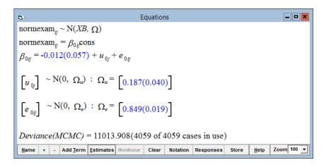
One first thing to note is that the level 2 variance estimate  $\sigma_{u0}^2$  here is larger than seen for the random effects model. This is because the SMVN coding in MLwiN has only been done for uniform priors and so any priors displayed on the **Equations** window should be ignored. A uniform prior for the variance will give a larger posterior mean estimate than a  $\Gamma^{-1}(\varepsilon, \varepsilon)$  prior as has been discussed in earlier chapters.
