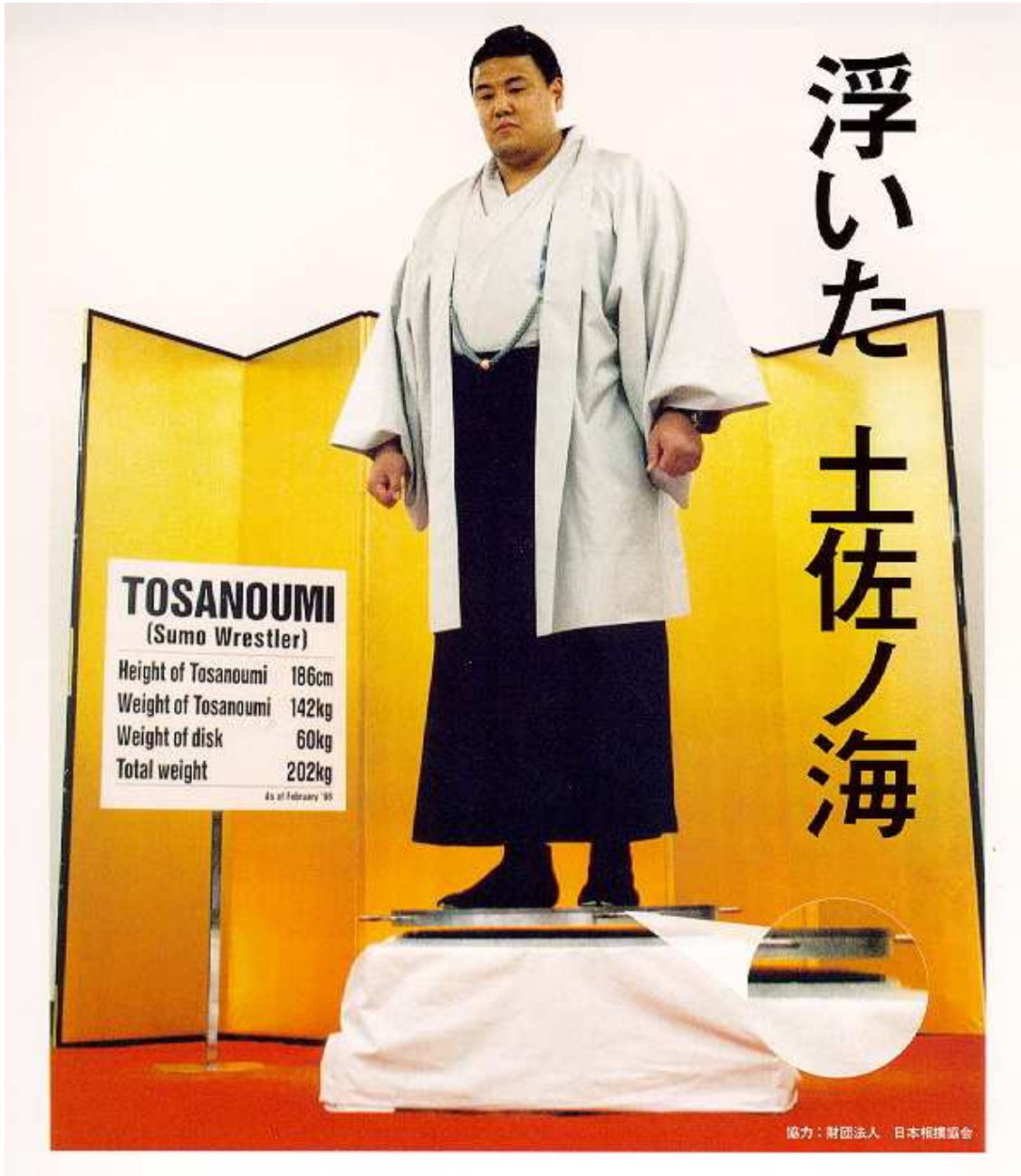
Figure 1.2: A sumo wrestler stood on a piece of magnetic material levitated over a superconductor, taken from the Asian Technology Information Program (ATIP) website [20].
