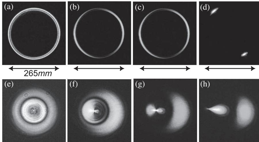
Figure 4.49: Photographs of the transition from (a,e) conical diffraction to (d,h) double refraction, as the incident beam is alligned away from the optic axis, in (a-d) the focal image plane and (e-h) the farfield, corresponding to the theoretical images in figure 4.35. The diameter of the rings, magnified onto a screen, is indicated.
