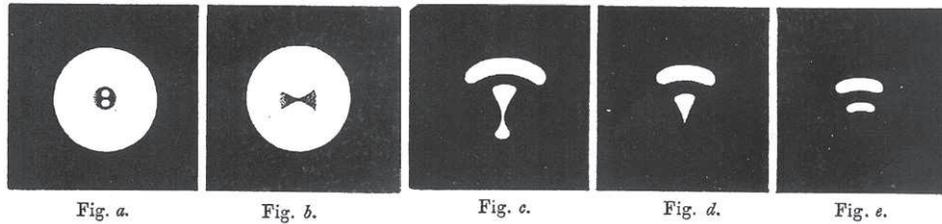
Figure 1.1: Lloyd's discovery of conical refraction: the transition from conical (a) to double (e) refraction, viewed through aragonite with a pinhole on the entrance face, illuminated by a distant lamp, reproduced from Lloyd (1837).
