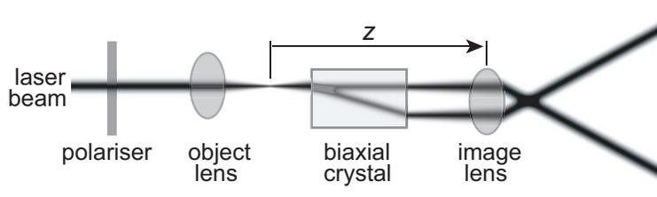
Figure 4.48: Observing conical diffraction: a collimated circularly polarised laser beam is focused through an object lens (focal length 70mm). The distance  $z$  is measured from the focus. A biaxial crystal of MDT (length 25mm), with faces cut perpendicular to its optic axis, refracts the beam, and the emerging cylinder (radius 0.4mm) is focussed by an image lens (focal length 6.4mm) onto a screen 2m away (image ring diameter 265mm).
