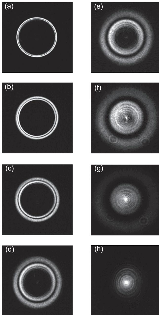
Figure 4.50: Photographs of the conical diffraction pattern from a 25mm slab of MDT, imaged at distances  $\Delta z = \zeta k_0 w^2$  equal to: (a)  $\sim 0$ , (b) 1.5, (c) 3.0, (d) 6.0, (e) 9.0, (f) 15.0, (g) 21.0, (h) 49.1, millimetres from the focal image plane. (The blemishes in the lower halves of (f) and (g) result from lens imperfections).
