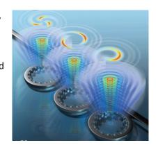
The Bristol invention is a novel way of generating light with OAM in a low cost and very compact form that enables integration on a chip. Large arrays of emitters, with different OAM states, can for the first time be fabricated with potential applications in chip to chip interconnect technology and more complex optical manipulation schemes in biophysics. The emitter can be tuned on the chip to emit specific OAM states, and also has the potential to work in reverse to detect specific OAM states.
