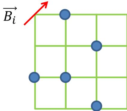
Hubbard model on a 2D grid with site-dependent magnetic field
