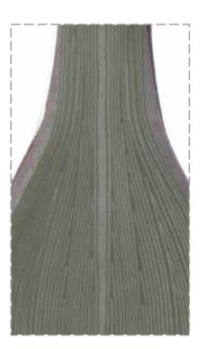
Surface scan shows well placed plies with good consolidation
