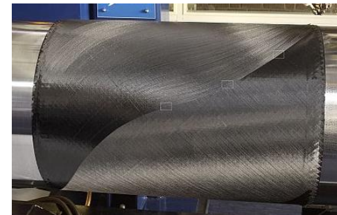
Variable fibre angle cylinder, optimised for bending [Delft]
