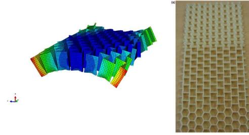
Gradient structures provide continuous variation of the mechanical and multiphysics behaviour of the material
