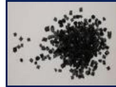
Recovered Dry Fiber and Pyrolysis Recovered Fiber Compounded with Polyetherimide (PEI)
