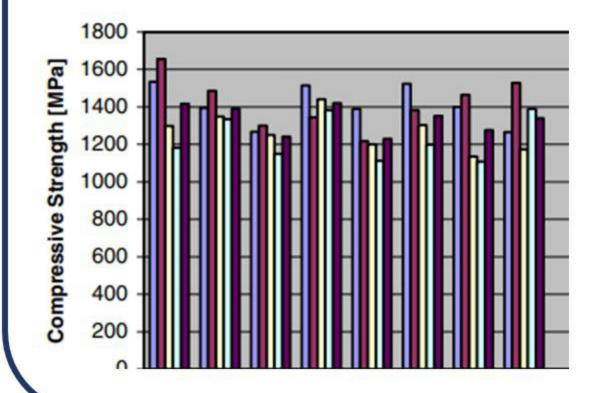
Round robin test: large variations were shown in compressive strength with the same material and testing method.
