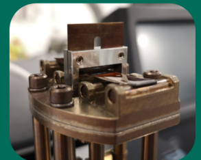
Figure 4: Razor applying true 3PB
