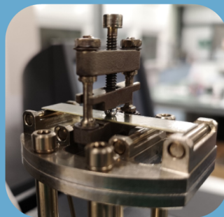
Figure 2: DMA 3PB bi-material beam experiment clamped in centre
