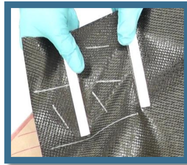
Apply shear prior to tool contact.
