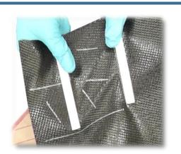
Preshearing is automated using a two part press
