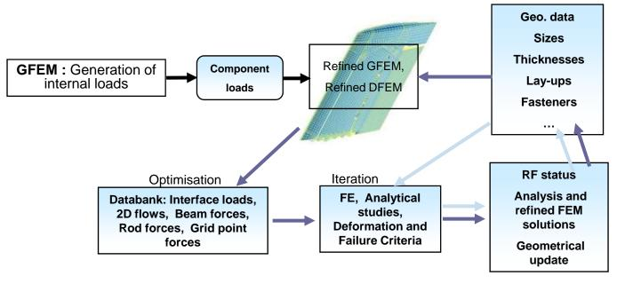
A Stress Process is required defining different level of analyses, e.g.
