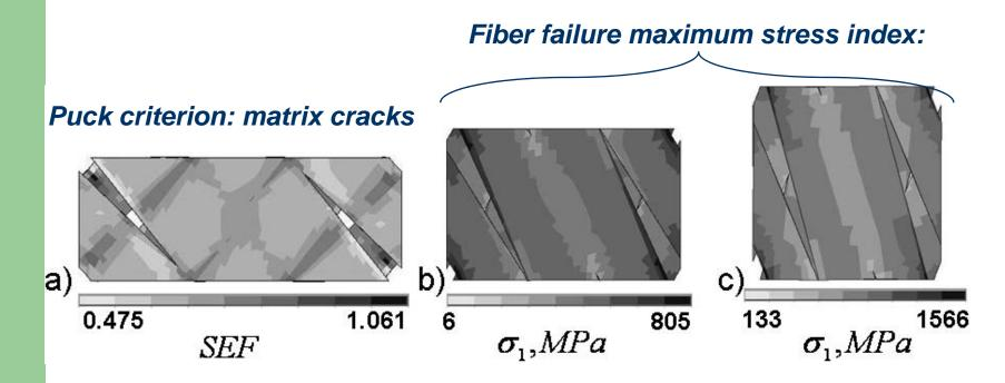
(a) Stress exposure factor (SEF) for ± 45° composite at applied deformation 2,1 %
