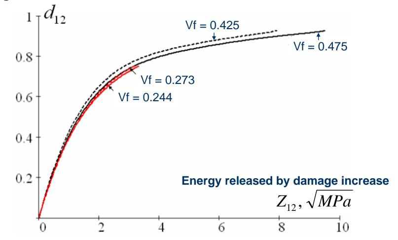
Almost does not depend on the fibre volume fraction!  $\Rightarrow$  convenient to use
