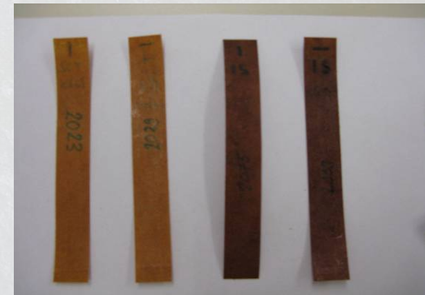
Samples for strap crush test
