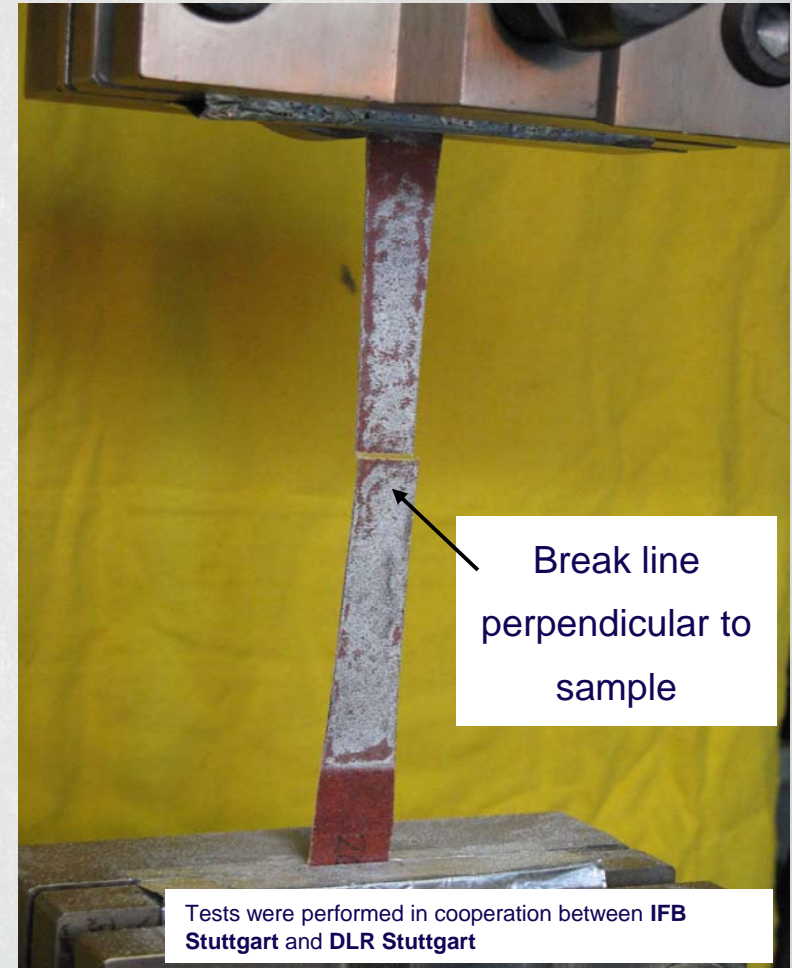
Broken test specimen
