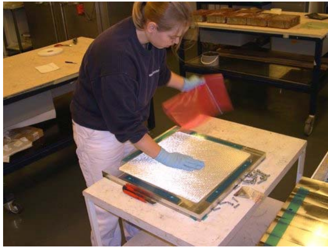
DTU specimens: Pre-pregs and vacuum assisted curing using an engaged double sided mould
