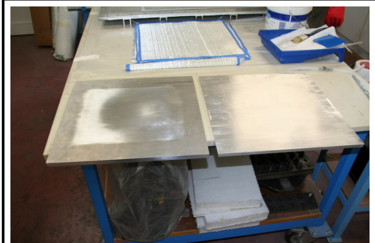
NTUA specimens: Hand lamination and vacuum assisted curing in single sided mould
