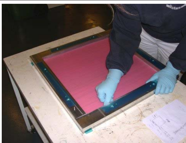
DTU specimens: Pre-pregs and vacuum assisted curing using an engaged double sided mould
